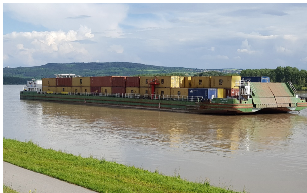
Fig.2: Motor freighter „Chan“ with container load on the Danube. When loaded with three layers, it carries 150 40'-containers of LNG (300 TEU)
