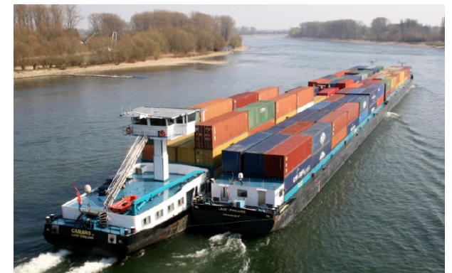
Fig. 4: Motor freighter boat and 3 push barges on the Upper Rhine. This set with a capacity of up to 600 TEU (300 40'-to-LNG containers) is suitable for the Danube.
